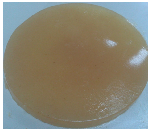
Fig. 1. Acrylated AbA-g-BC hydrogel synthesized at 30 kGy (H130, 0.3 mol of AA).
